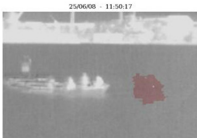
Photo 5. Infrared image of the MMA gas cloud near the floating cells
